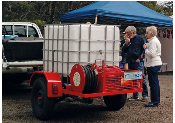
The Dolphin Sands community mobile fire pump
