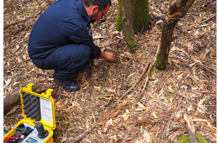
Checking fuel moisture in the path of the Riveaux Road fire so we can more accurately predict the fire's rate of spread
