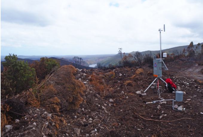
A Tasmania Fire Service portable automatic weather station installed at a remote location on the Zeehan complex of fires. Sometimes we walk or fly long distances into sites because there is not suitable road access
