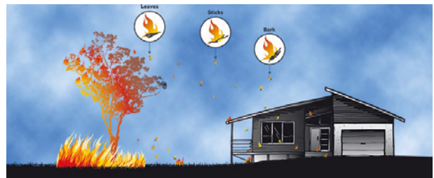
Embers ignite dry leaf litter in roof gutters
