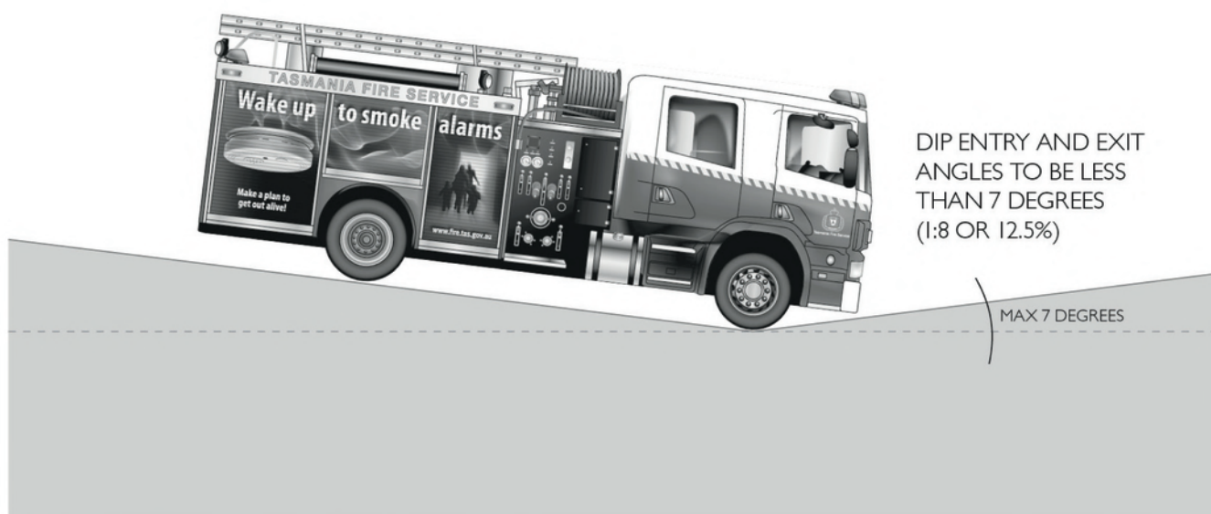
Figure 3 Dip approach and exit angles
